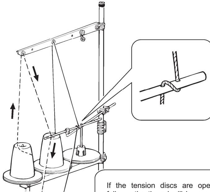
If the tension discs are opened as follows, the thread will become easier to thread.
