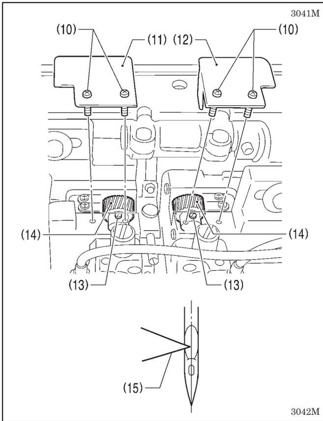
8. Loosen the screws (10), and then remove rotary hook base cover FL (11) and FR (12).
