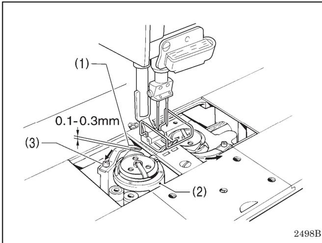
1. Loosen the set screw (3) and move the opener (1) to the left or right to adjust so that the clearance between the rotary hook (2) and the opener (1) is 0.1–0.3 mm when the opener (1) is pulled as far as it will go in the direction of the arrow.
