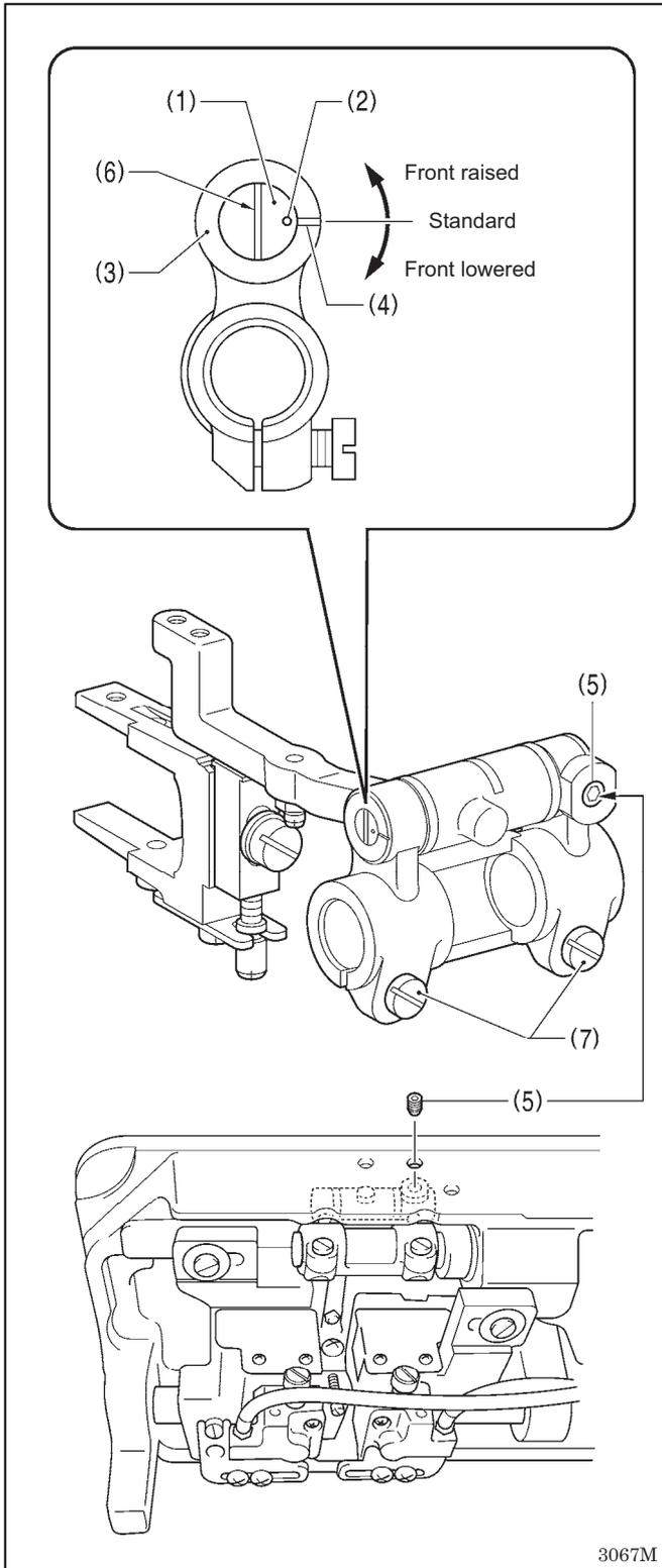
The standard angle for the feed dog is when the mark (2) on the feed bar shaft (1) is aligned with the reference line (4) on the feed rocker base arm (3).
