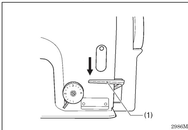
When the reverse lever (1) is pressed during sewing, the feed direction will be reversed. When it is released, the feed direction will return to normal.
