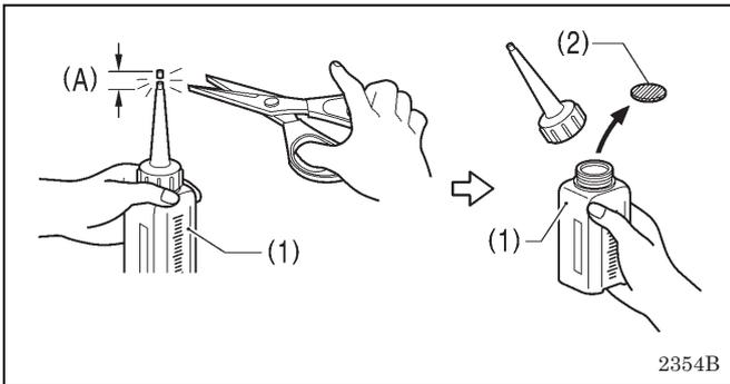
1. Hold the base of the nozzle of the accessory oil tank (1), and use scissors to cut about half-way along the straight section (A) of the nozzle.
