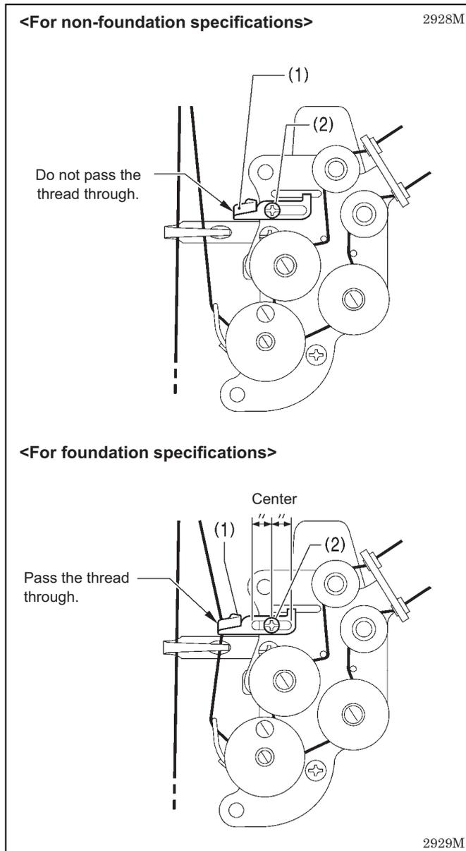
The thread take-up amount is adjusted by how the thread is passed through the thread amount adjuster (1).
