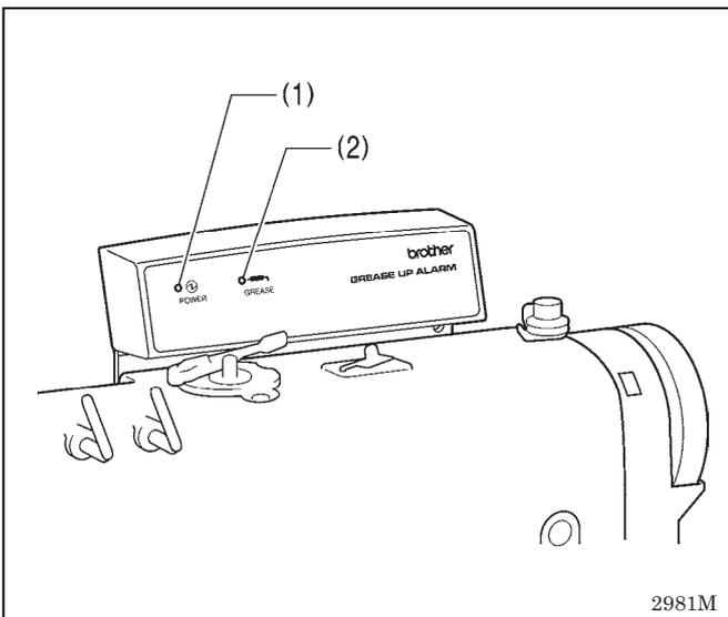
The alarm display is a device that shows the time until the next greasing is required.
