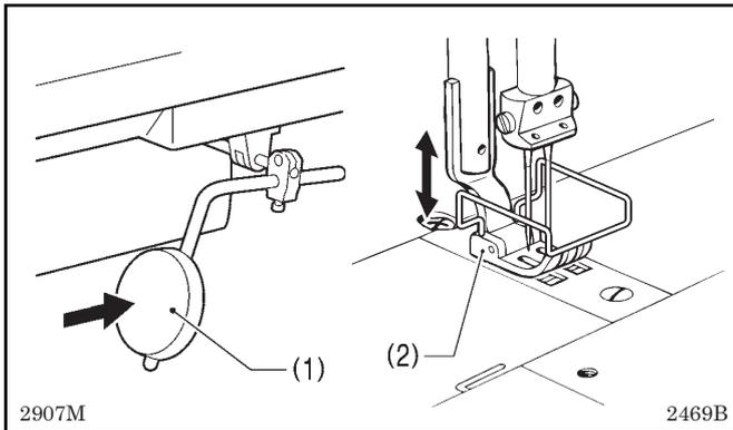
The presser foot (2) can be raised by pressing the knee lifter plate (1).
