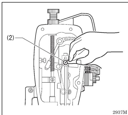
5. Use a cloth to wipe away any excess grease from around the screw (2).
