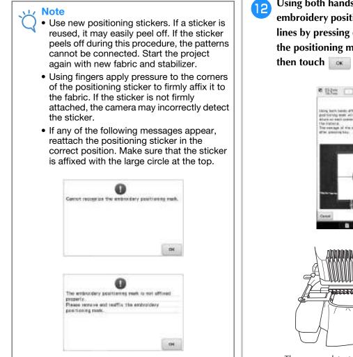
Using both hands affix the second embroidery positioning mark within the red lines by pressing down on each corner of the positioning mark onto the material and then touch
