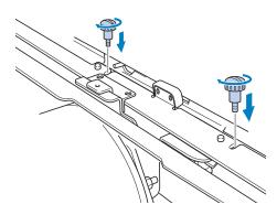
**7** While pushing in the cap frame driver toward the machine so that it is fully inserted, tighten the two lower thumb screws to secure the cap frame driver.
