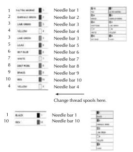
Since the thread colors on needle bars 2 to 10 will be used again after the thread spools are changed, they will not be replaced. However, different colors are assigned to the other needle bars.
