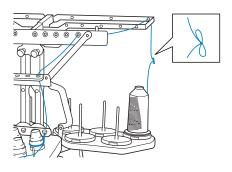
Pull out the old thread just after the needle bar thread guide.
