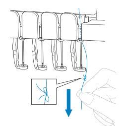
Continue pulling the thread until the knot is above the needle. Cut the knot.
