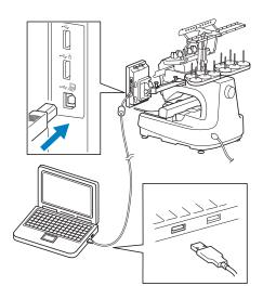
If the machine is positioned at a distance that prevents the USB cable from reaching the computer, embroidery patterns can be transferred from the computer by temporarily saving them on USB media or an SD card, which is then inserted into the machine. (Refer to "Saving embroidery patterns to USB media/SD card" on page 161.)
