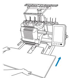
**5** While looking below the table, lightly lift it up, and then lower it so that the screw fits into the notch at the front of the guide plate.
