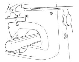
Pass the USB cable through the front USB cord clamp, and then close the clamp to secure the cable.
