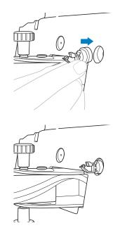
As described in steps 1 through 3, remove the protective cap from the rear screw hole on the side of the machine, and then insert an opened USB cord clamp.
