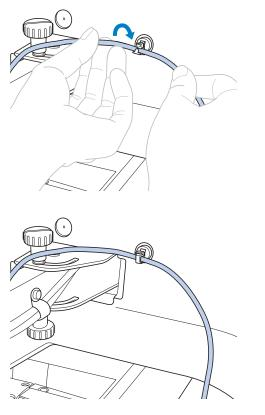
Using the same operation described in step **5**, secure the USB cable with the rear USB cord clamp. 8 Arrange the USB cable between the USB cord clamps so that the cable does not interfere with the operation of the machine.
