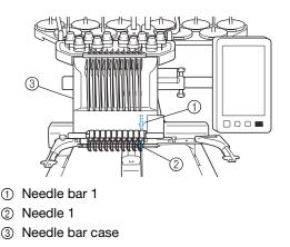
The machine automatically assigns a thread color to each needle. There are two methods for assigning the thread colors. With the automatic method (default method when the machine is purchased), needles that are already threaded with a color that will be used in the next pattern are assigned to the same thread color based on the needle bar assignments from the previous pattern in order to reduce the number of thread spool changes.
