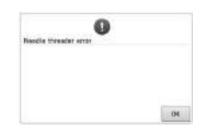
The automatic needle-threading mechanism did not operate correctly. Remove the thread entangled in the automatic needle-threading
