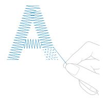
• If the stitches cannot be cleanly removed, trim the thread with scissors.
