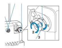
Pass the end of the thread through the guide 7 slit in the bobbin winder seat, and pull the thread. The cutter will cut the thread.
