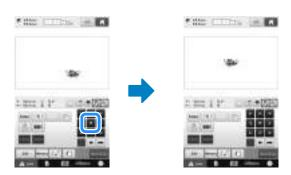
The pattern can also be moved by dragging it. If a USB mouse is connected, move the mouse to position the pointer on the desired pattern, and then while holding in the left mouse button, drag the pattern. The pattern can also be dragged by selecting it directly in the screen with your finger or the touch pen.
