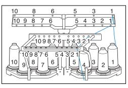
Pass the thread of a specified color through the holes on the thread guide, making sure that you have the thread color matched to the coordinating needle bar.
