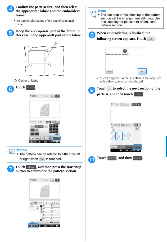
Hoop the fabric for the next design section aligning on the alignment stitching. In this case, align the left side of the hoop on the right side of the design section embroidered in step <sup>6</sup>.
