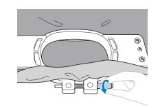
→ If the screw was tightened using a disc-shaped screwdriver, use the included disc-shaped screwdriver to loosen it.
