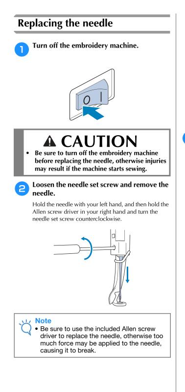
• Do not apply extreme force when loosening or tightening the needle set screw, otherwise the machine may be damaged.
