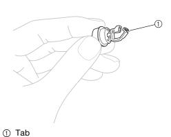
Hold the clip end of the USB cord clamp, and then firmly insert the other end into the screw hole where the protective cap was removed.
