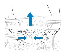
After the thread guide assembly support is 3 extended and the thread guide assembly is raised to its highest position, tighten the two thumb screws to secure the thread guide assembly in place.
