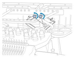
① Turn the screw counterclockwise three or four times to loosen it.
