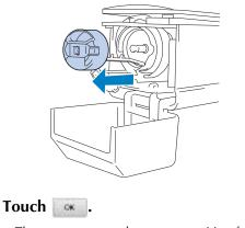
→ The race moves to the correct position for oiling.
