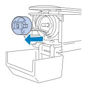
Use the included cleaning brush to remove З any lint and dust from the hook and its surrounding area.
