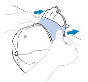
While pulling the lever toward you that is 15 located behind the handle on the right side of the mounting jig, rotate the cap frame to the left. After the cap frame has been rotated 90°, release the lever to lock the cap frame in place.
