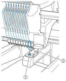
Needle hole in the needle plate
