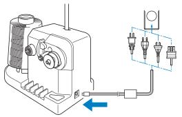
• Be sure to firmly insert the plug on the AC adapter into the DC input connector of the bobbin winder.
