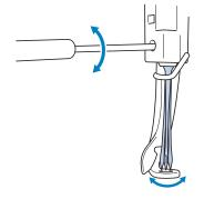
**3** With the flat side of the needle toward the back of the machine, insert the needle all the way up until it touches the needle bar stopper.
