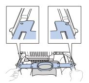
• The inner frame should be on top.
