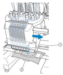
Needle at the embroidering position The needle is positioned over the hole in the needle plate 2.
