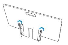
Position the table so that the notch at the center aligns with the machine bed, and then place the table flat on the guide plates.
