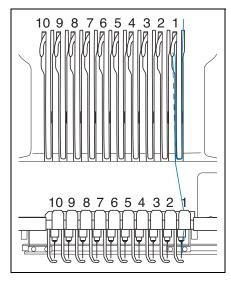
Pass the thread along the number 1 slot to pass it through the number 1 take-up lever hole from right to left.
