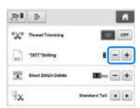
• A value between 1 and 8 can be specified. For example, if 3 is specified, sequential 3 jump codes will be converted to the trim code. But sequential 2 jump codes will not be converted to the trim code, it will be sewed as the feed (jump) stitch.
