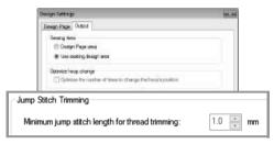
Specify the minimum jump stitch length for thread trimming.
