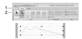
2. Drag the handle to adjust the selected pattern(s) to the desired size.
