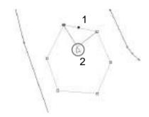
If the point is deleted, the corner is removed. Click the point (1), and then press the **Delete** key, or click 2.
