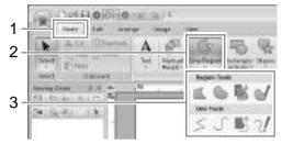
: Click points to draw a closed line constructed of straight lines.
