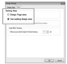
**Design Page area**: The patterns will be sewn so that the needle position when you start sewing is aligned with the center of your Design Page.
