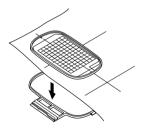
Keeping the reference lines on the embroidery sheet aligned with the reference lines for the first pattern section, place the fabric and inner ring of the embroidery hoop into the outer ring of the hoop, and then pull the fabric so that it is tight.
