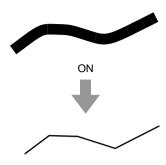
To replace the black lines with figure handle lines following the border of the outlines, clear the **Thinning Process** check box.
