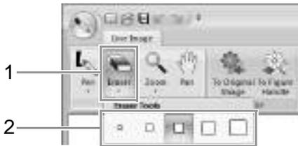
Select an Eraser tool according to the size of the area or thickness of the line to be erased.
