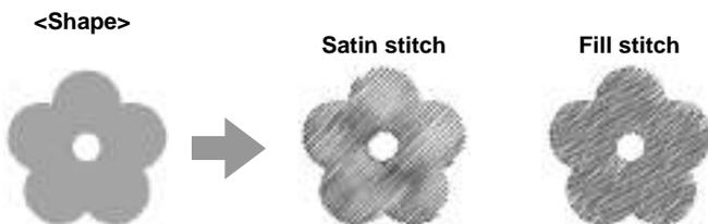
If a manual punching pattern is created using the above image as a guide, the stitching will appear as shown below.
