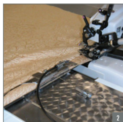
1. 1-Thread blind stitch including puller transport
